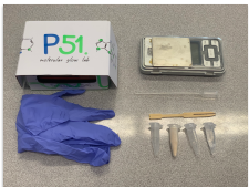
Fig 4. Field Test Kit: 4 x 1.5 ml mini-centrifuge tubes, pipette, 0.01g pocket scale, P51 viewer, gloves, sample collection toothpick.
