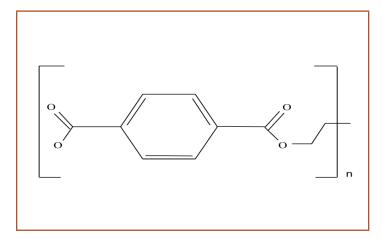
**Figure 2.** Polymer structure of (poly)ethylene terephthalate, where n is the number of times this polymer structure is repeated
